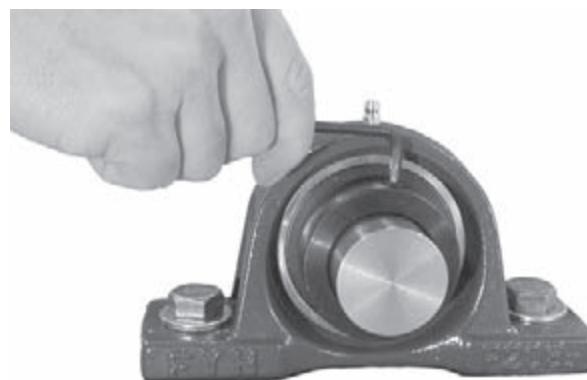
Fig. 14.10 Installing eccentric locking collar
