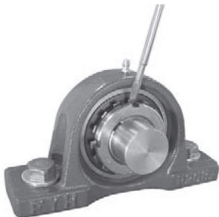
Fig. 14.8 Bending claw of washer (Locking locknut)
