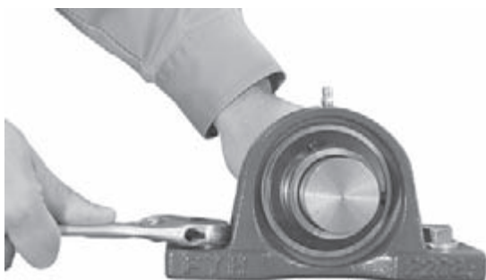
Fig. 14.4 Installation of setscrew units
