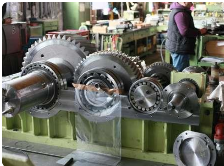
Parallel shafts in reduction units
