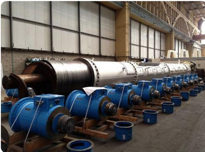
Pinion shaft sub-assembly
