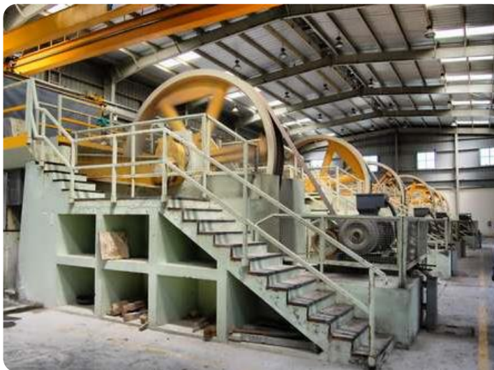
Multi blade gang saw machines for marble cutting
