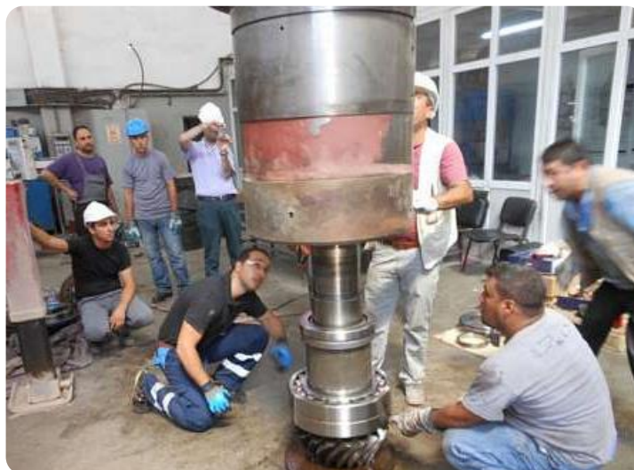
Reducer shaft of cement crusher
