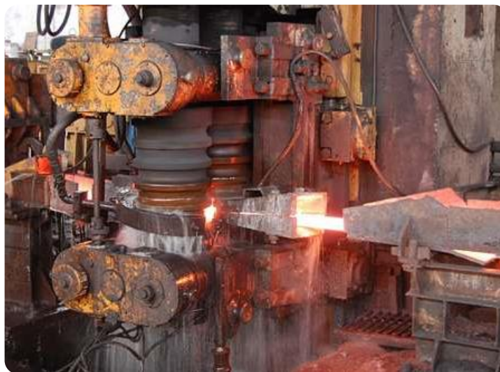
Rebars rolling mill stand horizontal stands and vertical stands
