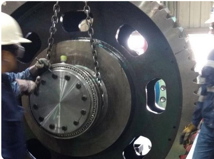
Speed reducer of hot-strip rolling mill stand
