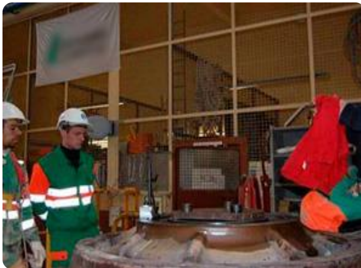
Vertical pre-crusher for cement production
