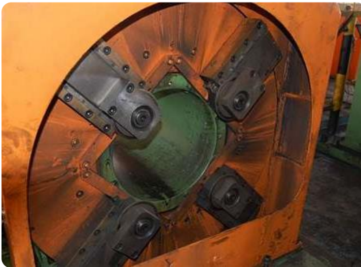
Pipe rolling mill cutting head
