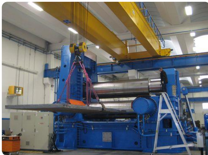
Variable axis plate bending machine
