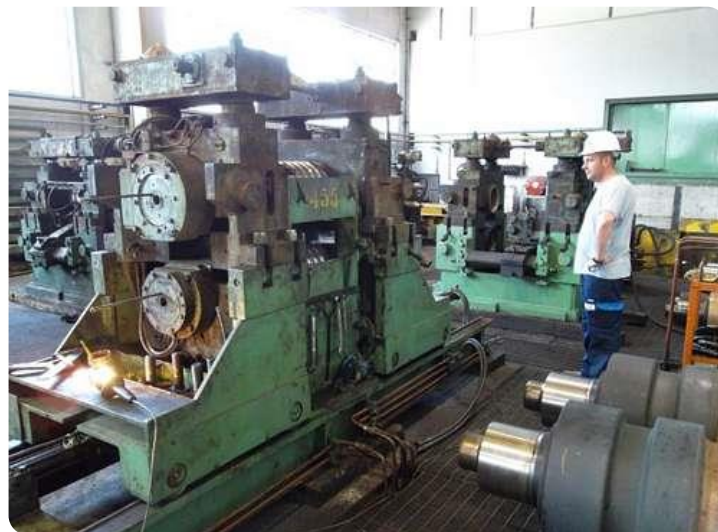
Hot rolling mill (roughing)
