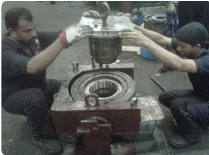
Beam mill stand for Angles (L-shaped cross-section)
