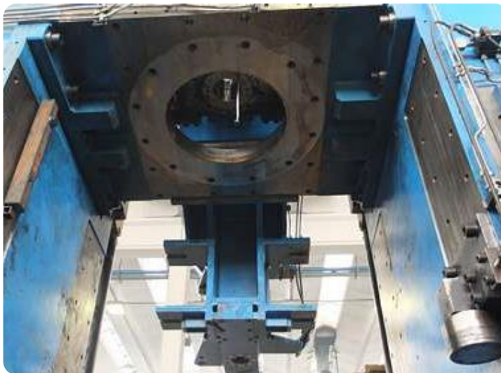
High reversible hot finishing mill stand for pipes
