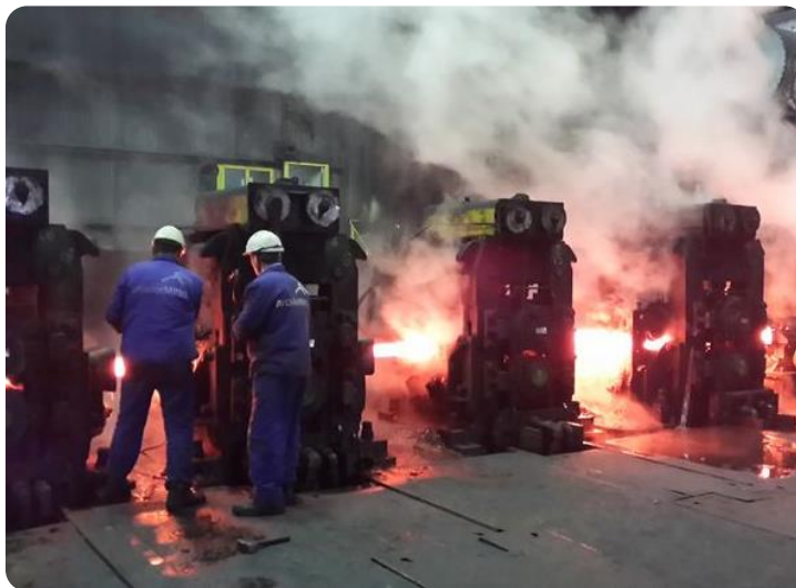
Wire rolling mill
