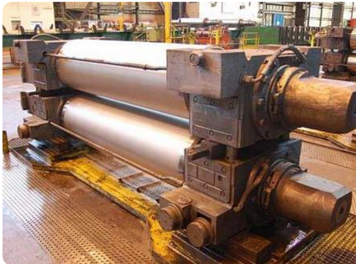
Cold rolling mill
