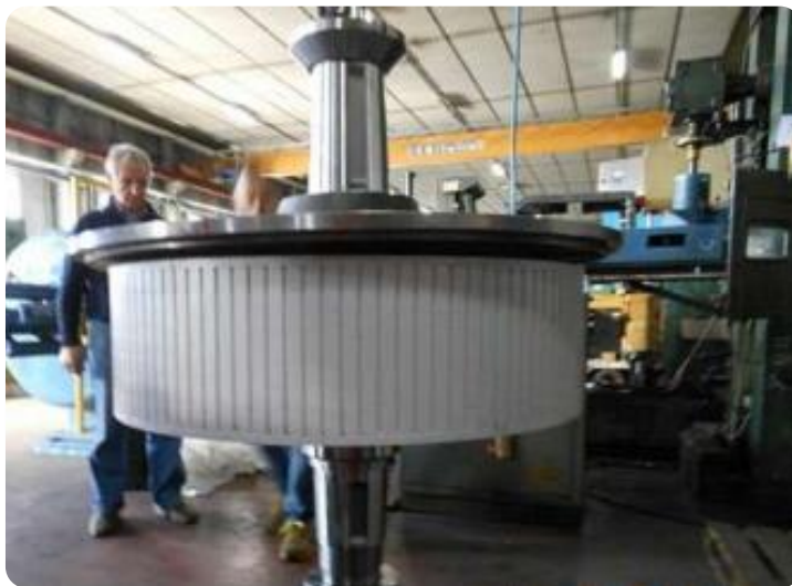
Wind mill main rotor
