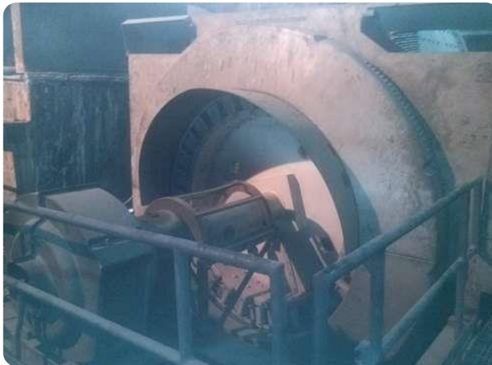
Ball mill pinion gear for copper production
