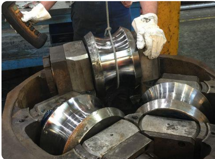
3-roll stretch reducing mill for the production of seamless tubes
