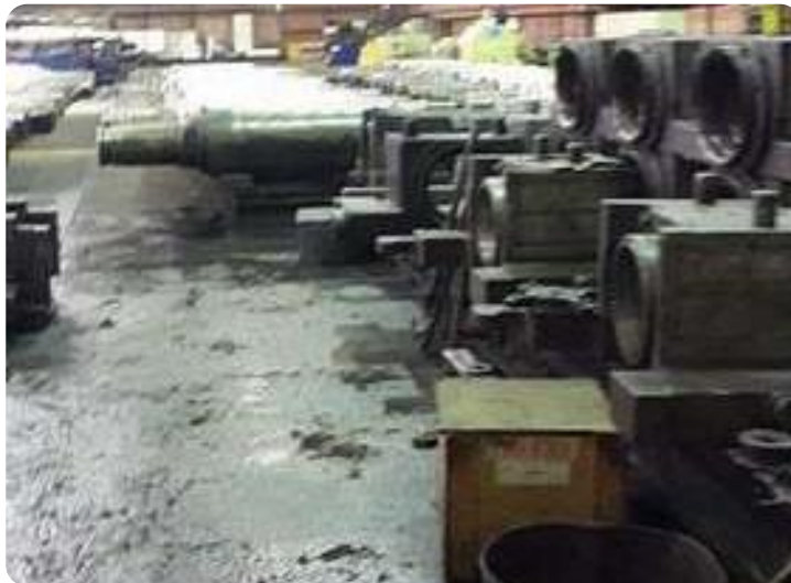
Work roll of tandem mill
