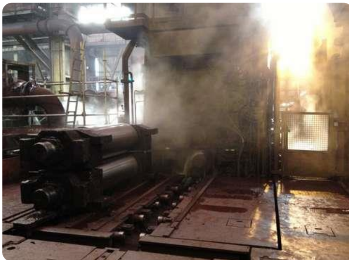
High speed finishing stripping mill
