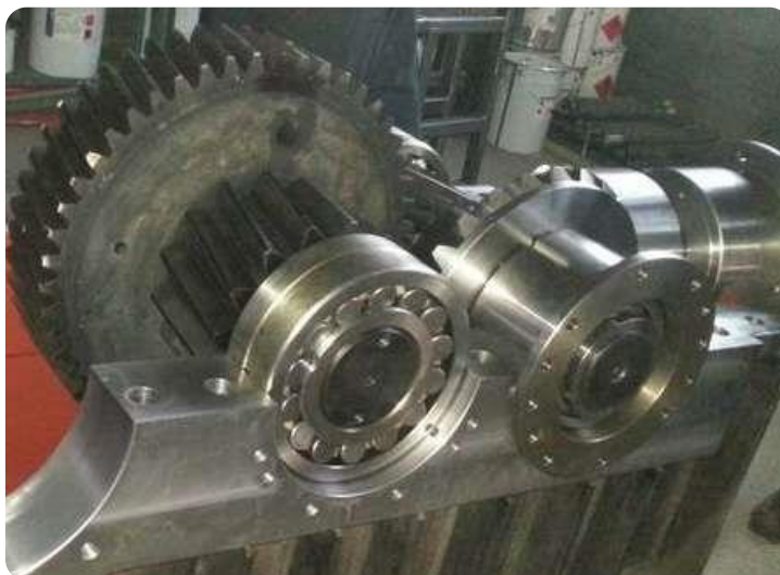
Gearboxes for main drive of transportation system for coal
