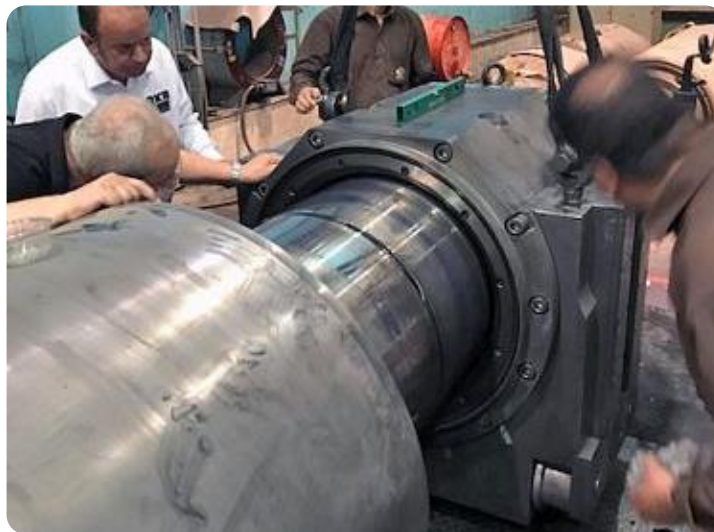
Back-up roll Danieli FATA Hunter cold rolling mill (Aluminium)
