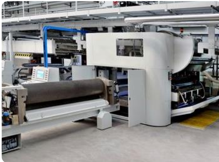
Cartridge for corrugator machine
