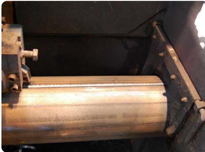
Pipe welding machine (OTO Mills)
