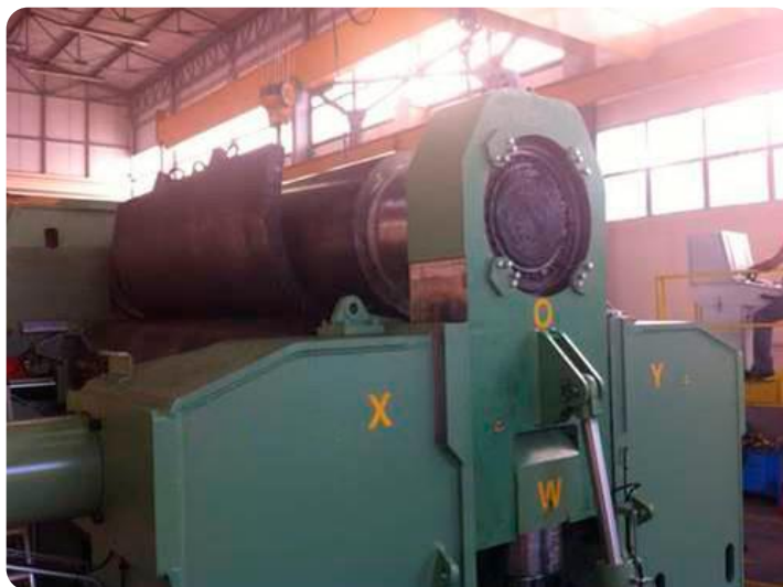
Variable axis plate bending machine
