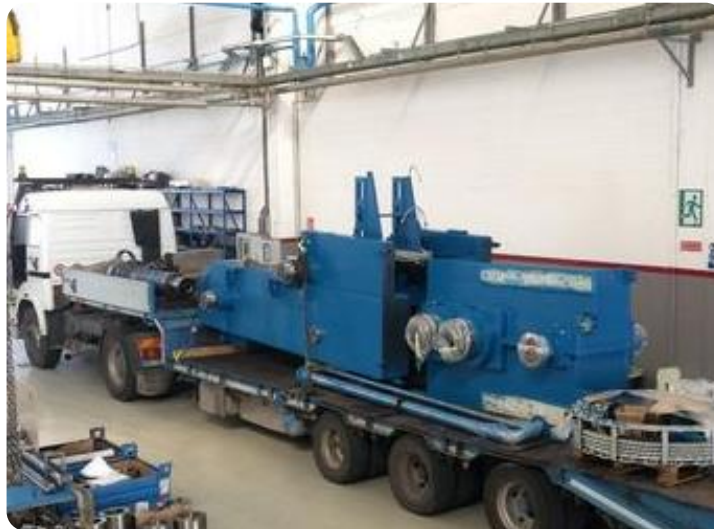
Gearbox Pomini Farrel for Riva cage 8, main pinion bearing
