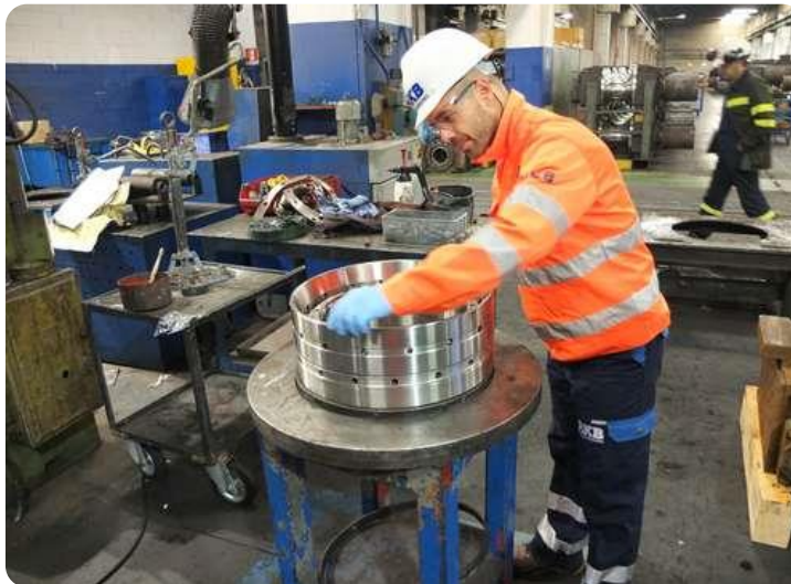
Finishing 2Hi stand for rolling mill MPM
