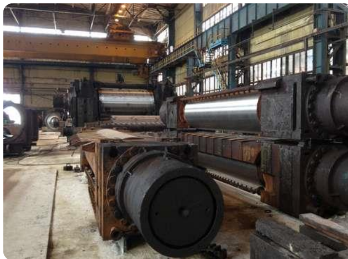
High reversing hot finishing mill stand
