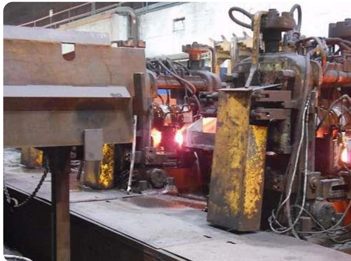
Rolling mill for steel reinforcing bars
