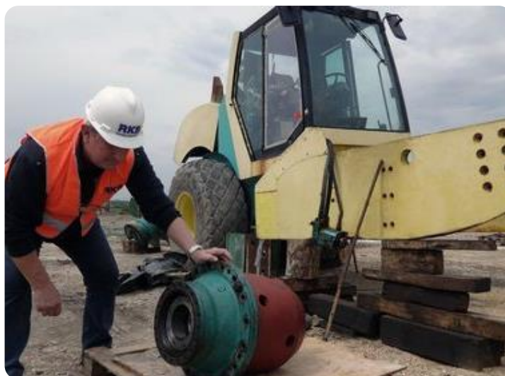
Single drum vibratory roller for soil compaction
